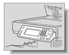
3 To return the control panel to the upper position, pull the control panel release lever toward you, and then pull up on the control panel.
